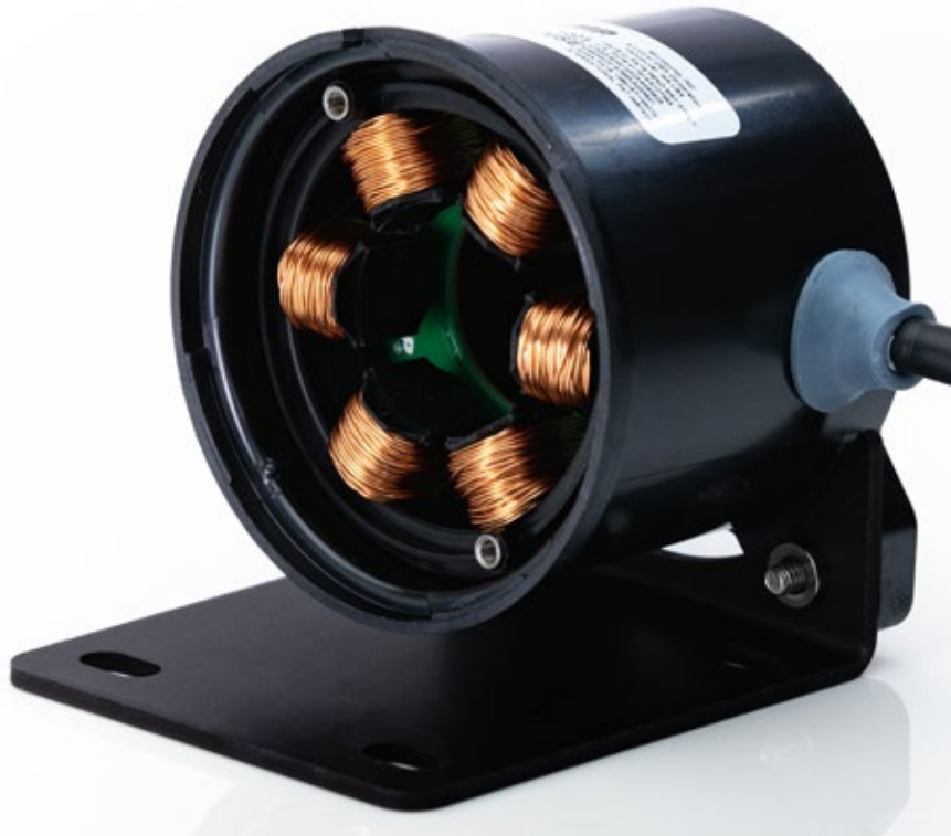
EagleDrive™ DEMSE Brushless DC Motor | SE mount 10-38 VDC | 250-8,000 RPM 70.62 mNm Torque (max)
