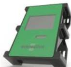
Steam trap and machine health monitoring with batteryless sensors that use only harvested energy.
