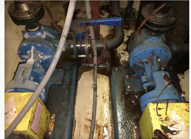
Packed pump at right leaking cocoa butter, O-ring sealed pump at left with no leakage.
