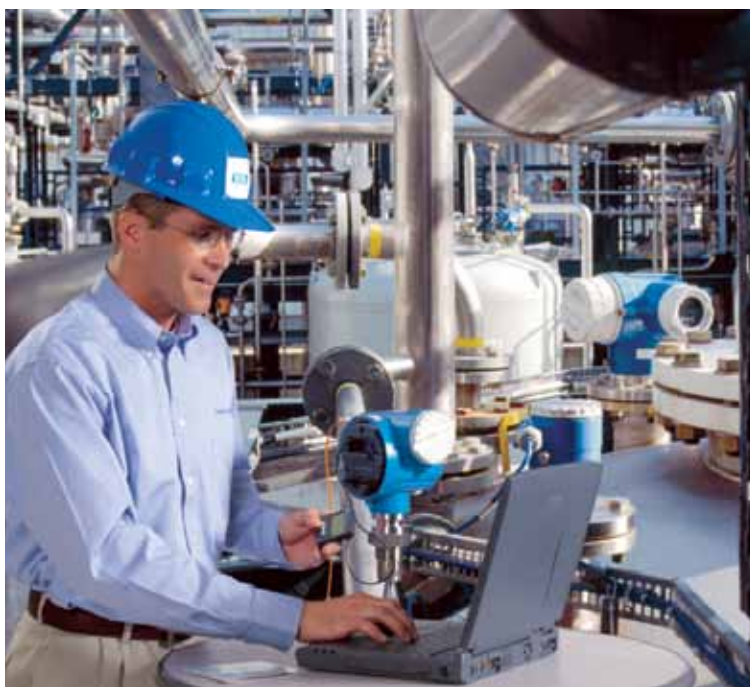
Figure 2. A technician manages a flowmeter's calibration data via a software system, such as Endress+Hauser's CompuCal calibration management system.
