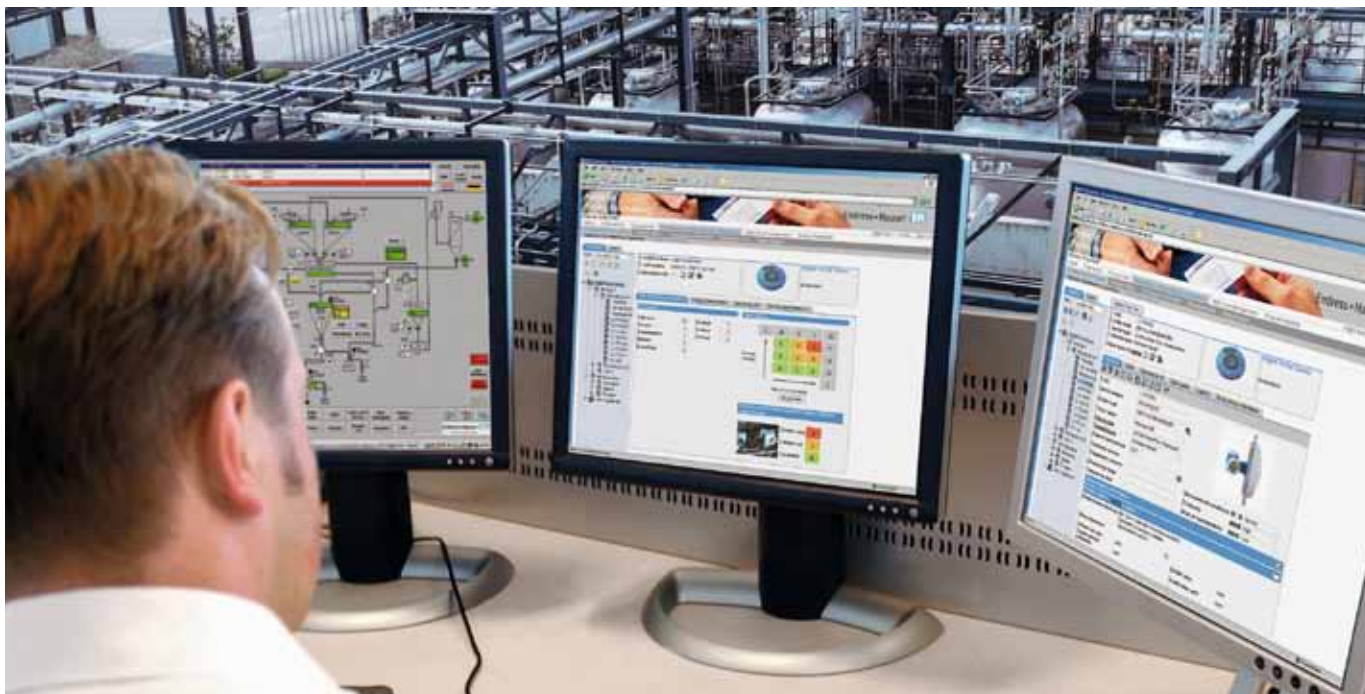
Figure 1. Flowmeter calibration data stored in an asset management system, such as Endress+Hauser's W@M Life Cycle Management System.
