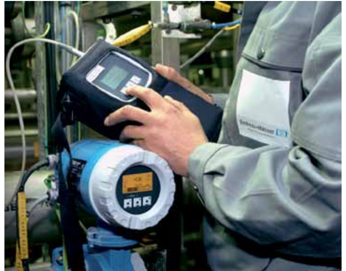
Figure 7. On-site flow verification performed with a test and simulation device - removal of the instrument from the pipe is not required.
